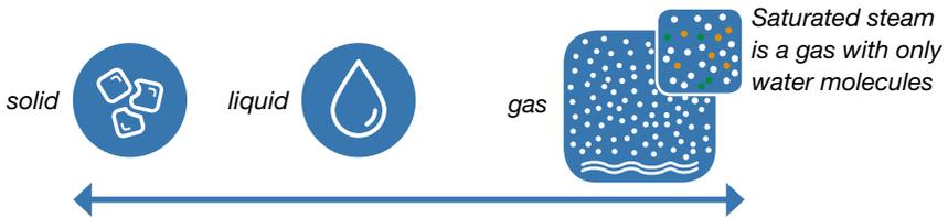
Definition of saturated steam EN 285:2015 clause 3.27: water vapour in a state of equilibrium between its liquid phase and its gas phase.
